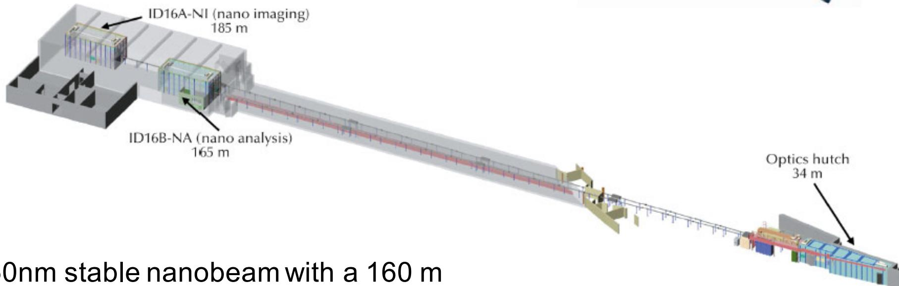
60nm stable nanobeam with a 160 m focalization length
