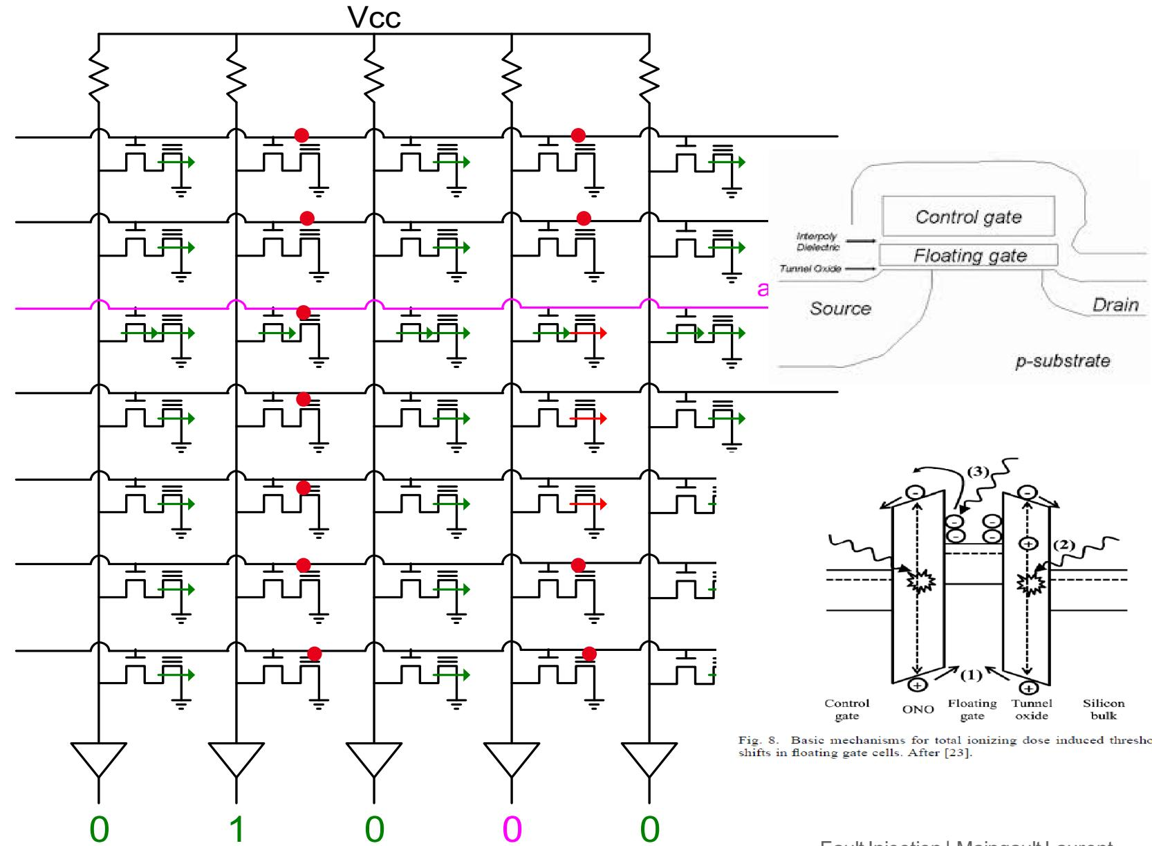
Fig. 8. Basic mechanisms for total ionizing dose induced threshold voltage shifts in floating gate cells. After [23].
